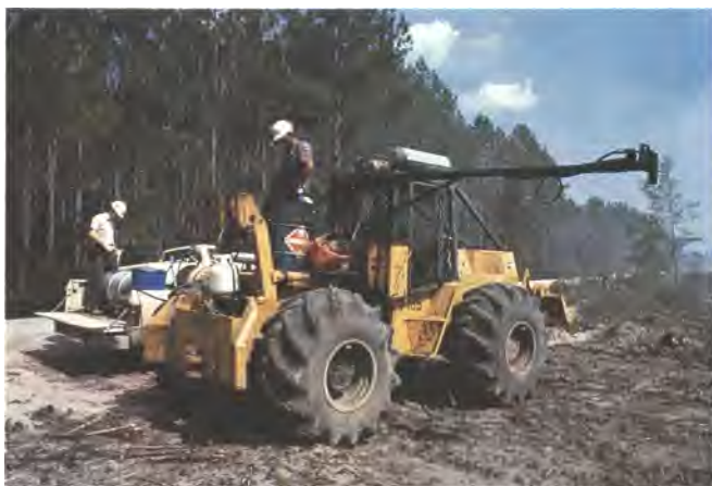
Tractor-mounted firing device for piled-debris ignition
